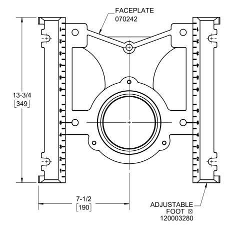
☑ RECOMMEND FEET BE SECURED TO FLOOR WITH 1/2" BOLTS AND ANCHORS (BY OTHERS).
