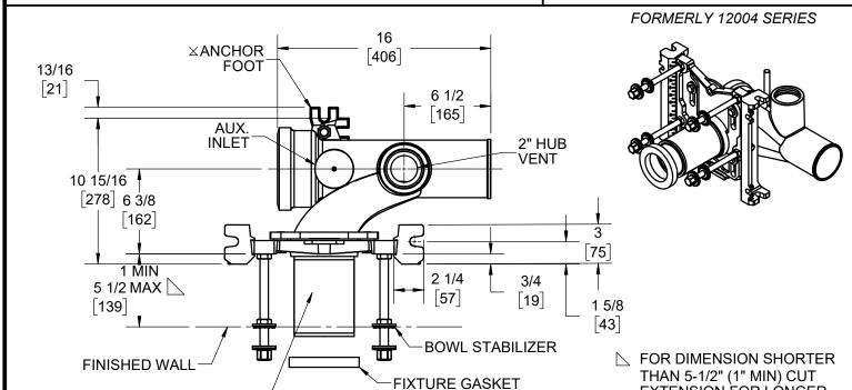
✓ RECOMMEND FEET BE SECURED TO FLOOR WITH 1/2" BOLTS AND ANCHORS (BY OTHERS)
