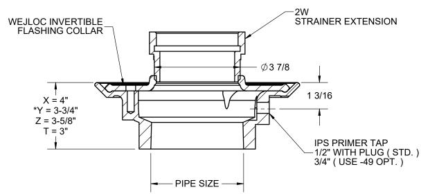
\*GASKET ON -Y CONNECTION CONFORMS WITH ASTM-C564
