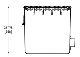
CHANNEL BRACKET AND OUTLET ASSEMBLED TO CATCH BASIN ON-SITE AT LOCATIONS NEEDED.
