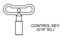
CONTROL KEY USED TO OPEN COVER AND OPERATE HYDRANT
