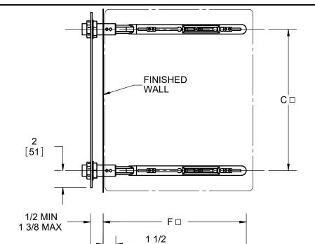
☐: VARIABLE DIMENSION. DEPENDS ON FIXTURE. STANDARD ADJUSTABLE SLEEVE IS 4".
