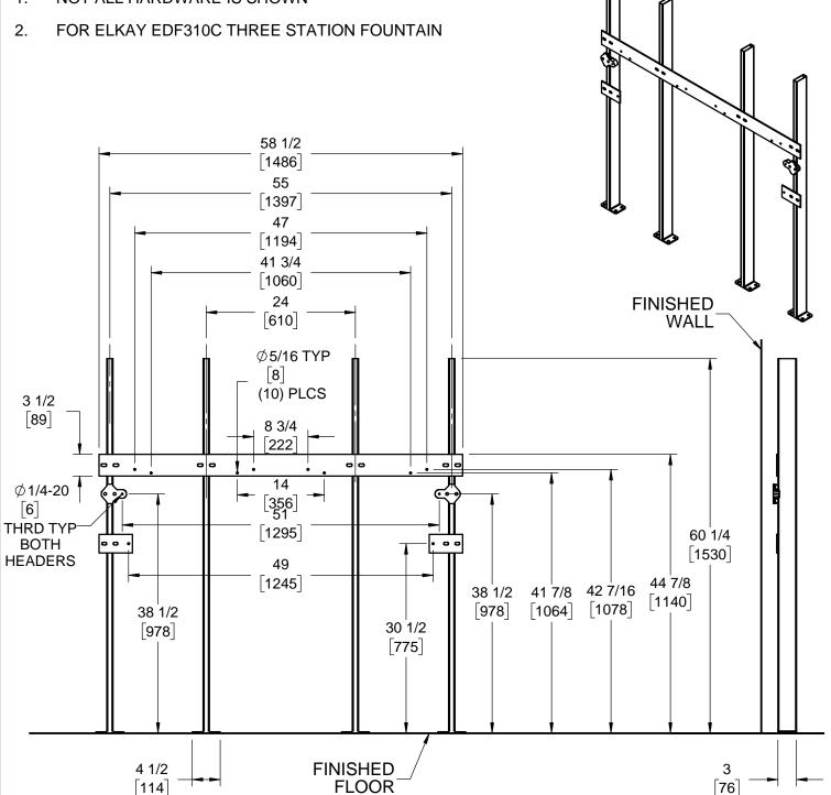
JOSAM RECOMMENDS - FEET BE SECURED TO FLOOR WITH 1/2" BOLTS AND ANCHORS BY OTHERS
