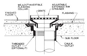
30000-E1 Series Adjustable Strainer Floor Drain shown installed in a concrete finish floor of two-pour construction. Extended rim protrudes 1 inch above finish floor and serves as a receptacle for the emptying of liquids.
