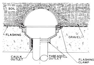
39600 Series Planting Area Drain shown in a typical installation providing drainage for an indoor planting area. Stainless mesh screen covered dome prevents entrance of dirt and gravel at the base of the planting area.
