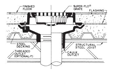
32100-81 Series SUPER-FLO $^{\circ}$  Floor Drain shown installed in a medium-duty single-pour concrete floor supported by steel construction.
