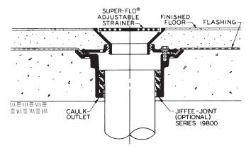
30000-A Series SUPER-FLO<sup>®</sup> Adjustable Strainer Floor Drain shown installed in a concrete finish floor of two-pour construction. The versatile JIFFEE-JOINT Gasket makes the caulk connection to the drainage line.
