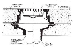
32100-AE-81 Series SUPER-FLO® Floor Drain shown installed in a poured concrete floor with floor finish. LEVELEZE® Adjustable Collar provides vertical adjustment, facilitating installation and forming a perfect surface between top of drain and floor finish.
