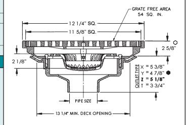
CONFORMS WITH ASTM-C564.
