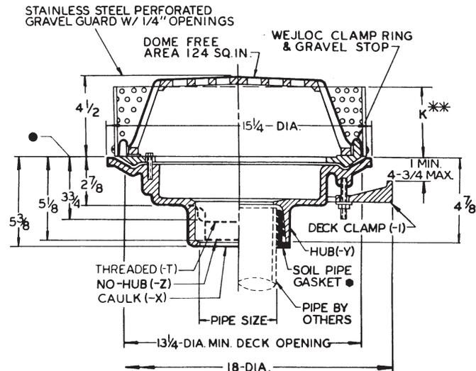
● CONFORMS WITH ASTM-C564.
