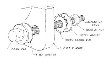
FH Hardware Part #: 565985T Mounting Stud and Back-up Nut not included in FH Hardware Kit. CARRIERS
