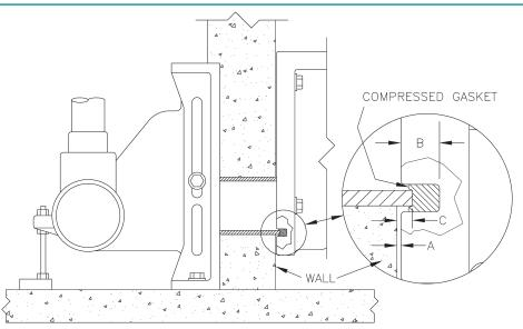
This is a side view. The enlarged inset shows the depth of the gasket within the groove of the fixture and the extension with proper pressure on the gasket.
