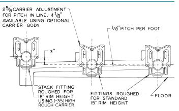
The above shows an installation utilizing a standard JOSAM stack fitting with the carrier on this fitting roughed for wheelchair use. With this installation one to three horizontal fittings can be connected to the stack fitting.
