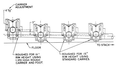
To the left is a possible installation utilizing the -35 Option at the end of a battery of standard rough carriers.
