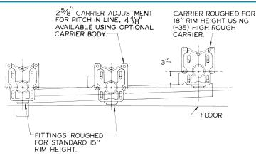
The above shows an installation utilizing a JOSAM vertical fitting and carrier and a horizontal waste line with fittings and carriers. The horizontal fitting and carrier on the end show the (-35) high rough for wheelchair use.
