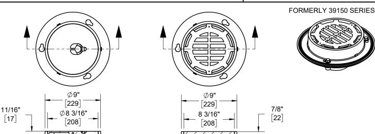
BODY WITH SOLID BRONZE GROUND JOINT PLUG WITH LIFT RING
