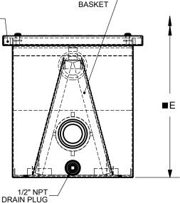
■ MINIMUM HEIGHT REQUIRED FOR REMOVAL OF SOLIDS BASKET. IF "-EXT " OPTION IS SUPPLIED, ADD EXTENSION HEIGHT TO THIS DIMENSION.
