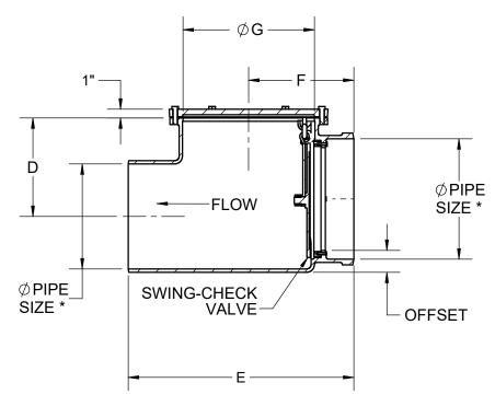
\* HUB & SPIGOT DIMENSIONS ARE IN ACCORDANCE WITH E.H.C.I. SOIL PIPE STANDARD.
