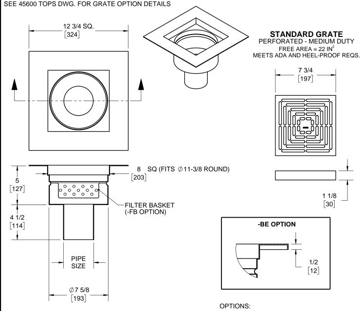
OUTLET O.D. DESIGNED TO FIT CLOSELY WITH I.D. OF NO-HUB CAST IRON PIPE
