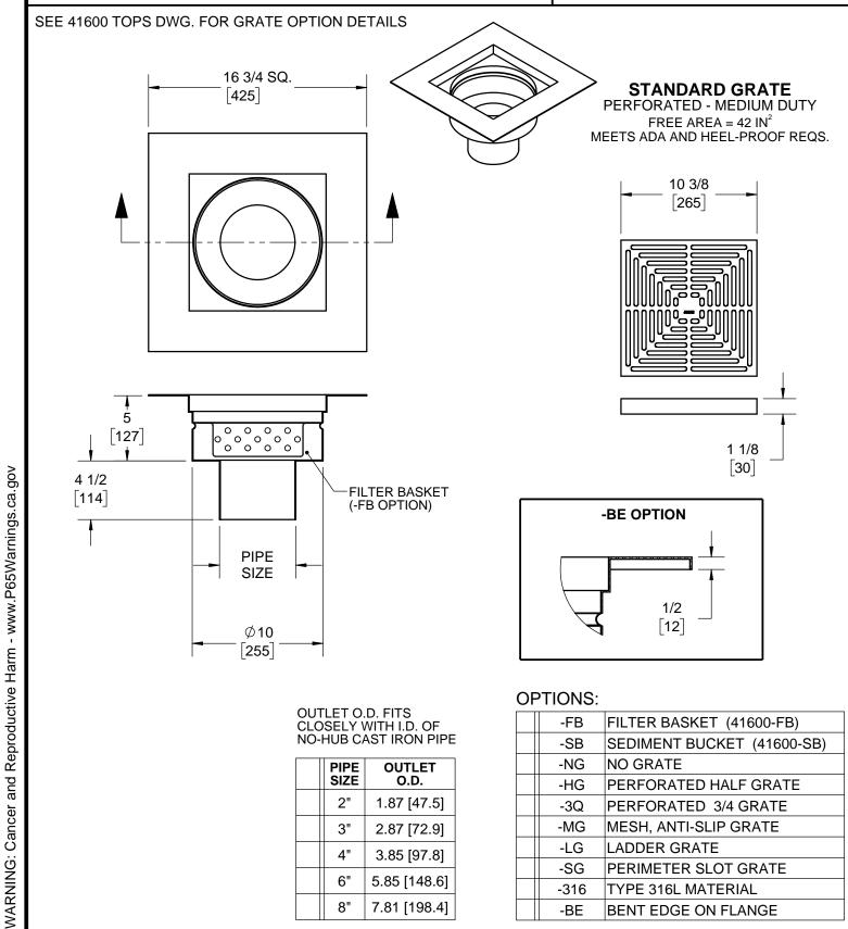
OUTLET O.D. FITS CLOSELY WITH I.D. OF NO-HUB CAST IRON PIPE
