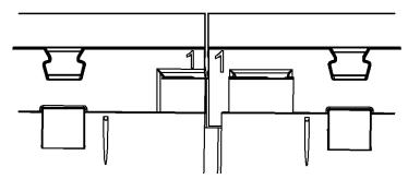
4) Lay out and orient the channel elements upside down in the proper sequence alongside the excavated trench (as per installation plan, if available). Give attention to the channel numbers. If the layout has a T connection or right angles, you must use "-T" channels as explained in the appendix. The –T modification allows for side connections. If the layout has MMS (Male Male Standard flow) or MMR-T (Male Male Reverse flow) channels they must be placed where the layout drawing shows.
