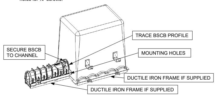
Flip over entire assembly. Support the catch basin with rebar or threaded rods. Secure BSCB to catch basin with hardware provided. Set channel and continue trench install.
