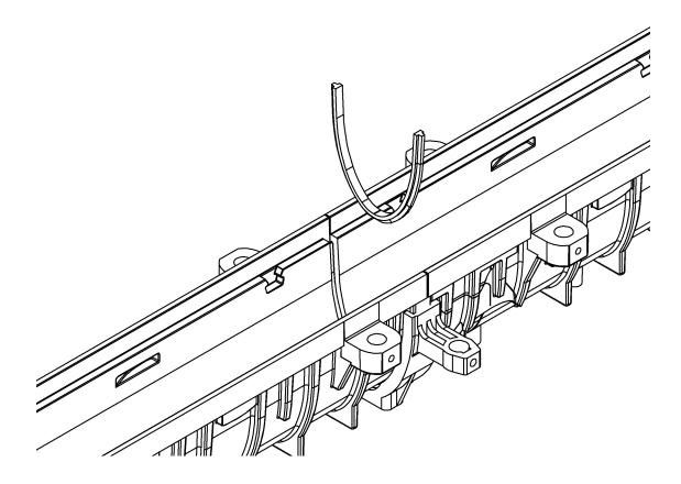
12) Clean any spilled concrete from gratings, channels, and outlet points. Remove plastic wrap from gratings. Insert and secure gratings to channel body using the appropriate grating locking system.
