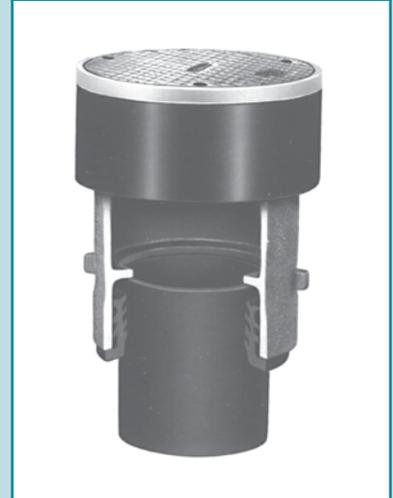
57000-Y Series KLEENATRON® Cleanouts feature JOSAM JIFFEE-SET connections with MULTI-TITE® service weight (SV) soil pipe gaskets in 2, 3 and 4 inch sizes for labor-saving assembly to service weight and no-hub cast iron pipe, and to PVC and ABS pipe. Merely lubricate gasket and pipe, set cleanout in place, push down until top of pipe contacts built-in stop and the joint is complete.
