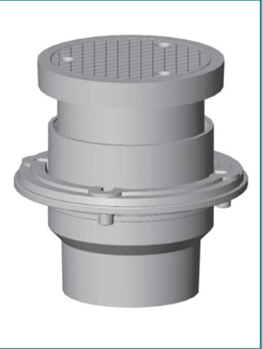
55000-Y Series KLEENATRON® Cleanouts feature JOSAM JIFFEE-SET connections with MULTI-TITE® service weight (SV) soil pipe gaskets in 2, 3 and 4 inch sizes for labor-saving assembly to service weight and no-hub cast iron pipe, and to PVC and ABS pipe. Merely lubricate gasket and pipe, set cleanout in place, push down until top of pipe contacts built-in stop and the joint is complete.
