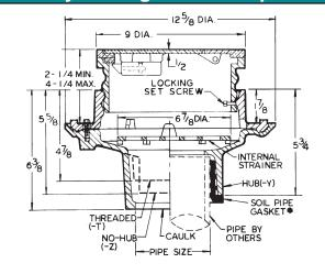
CONFORMS WITH ASTM-C564.
