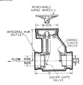
**NOTE:** SWING-CHECK VALVE NORMALLY HANGS IN CLOSED POSITION, BUT CAN BE SET TO HANG OPEN.
