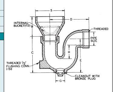
**NOTE:** WHEN (-51) FLUSHING CONNECTION IS USED, A VACUUM BREAKER SHOULD BE INSTALLED SUBJECT TO CODE REQUIREMENTS.
