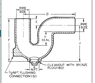
**NOTE:** WHEN (-51) FLUSHING CONNECTION IS USED, A VACUUM BREAKER SHOULD BE INSTALLED SUBJECT TO CODE REQUIREMENTS.
