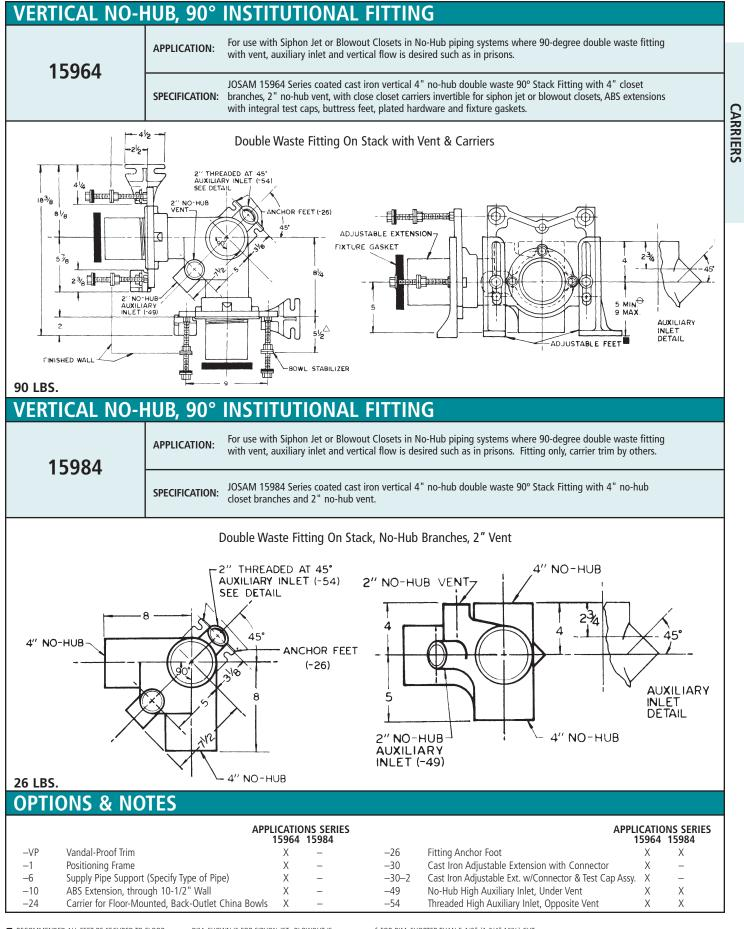
RECOMMENDED ALL FEET BE SECURED TO FLOOR WITH 1/2" BOLTS AND ANCHORS BY OTHERS. DIM. Shown is for siphon jet. Blowout is:  $\ominus$  11" min. & 16-1/2" max.
