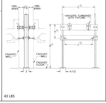
↔ VARIABLE – DEPENDS ON FIXTURE EXCEPT WHEN STD. PLATE IS FURNISHED. C=18-1/2 RECOMMEND ALL FEET BE SECURED TO FLOOR WITH 1/2" BOLTS AND ANCHORS BY OTHERS.
