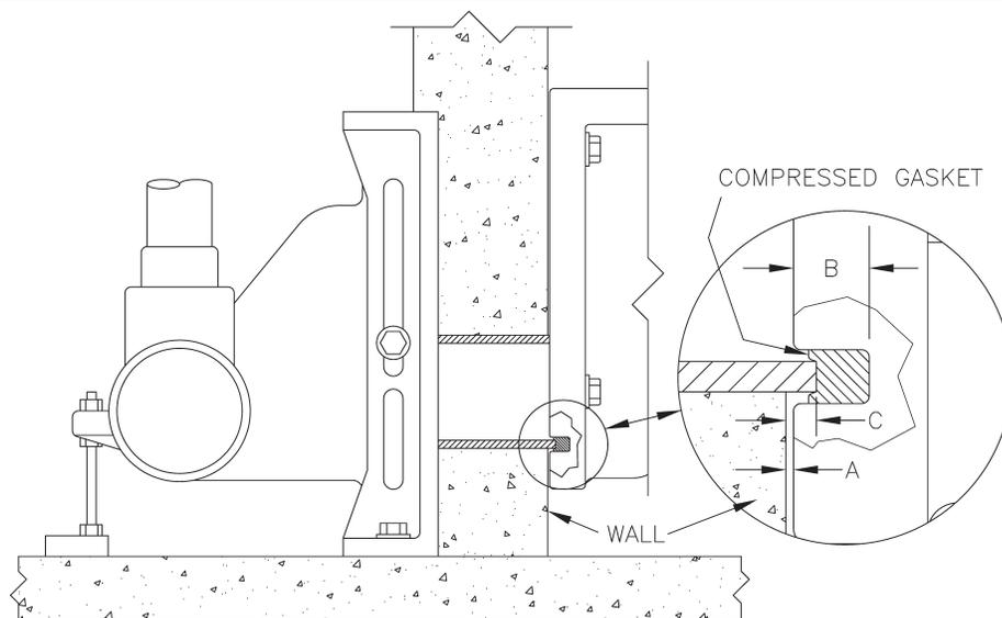
This is a side view. The enlarged inset shows the depth of the gasket within the groove of the fixture and the extension with proper pressure on the gasket.
