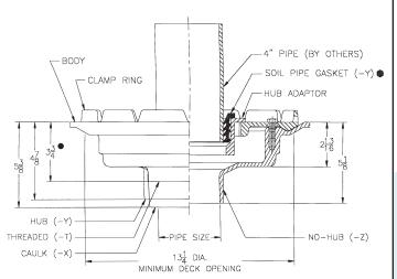
CONFORMS WITH ASTM-C564. THIS DIM. IS 5-3/4" FOR 23508-T.
