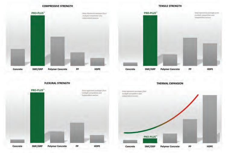
The unique properties of the PRO-PLUS<sup>™</sup> trench drain system allow for considerably less thermal expansion than polymer concrete, polypropylene, and high-density polyethylene.
