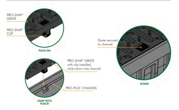
The PRO-SNAP<sup>™</sup> system constitutes another innovation for securing grates. The whole process has never been as fast or as simple. All of the different grate types can be secured and removed quickly and easily with a single hand movement, without the use of bolts or special tools.
