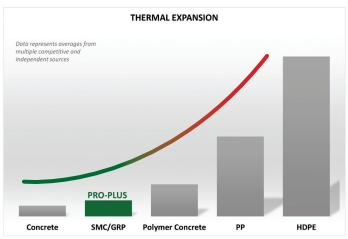
The unique properties of the PRO-PLUS® trench drain system allow for considerably less thermal expansion than polymer concrete, polypropylene, and high-density polyethylene.
